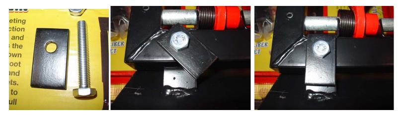
Find the brackets and bolts shown on the left picture. Find the notch on the back of the deflection plate, shown in the middle picture. Right behind the notch, there is a hole for the bolt to go into. Place the bracket down over the notch like shown in the right picture and tighten down the bolt/nut. The deflection plate is now in place and wont
