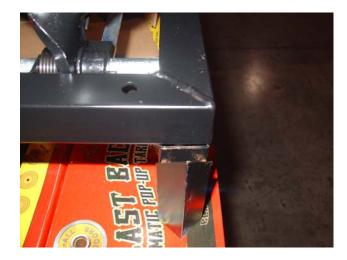
Start by finding the front of the Blast Back. The front has the legs angled outwards for deflection purposes. See above for left and right sides. At the top of the leg, there is a lip that goes upward, this is where the deflection plate will rest.
