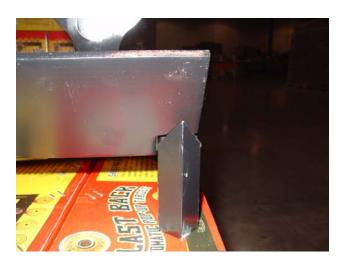
See above for how the deflection plate rests on top of legs. The deflection plate will rest in this position even without the brackets installed.
