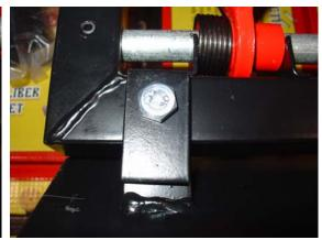
Find the brackets and bolts shown on the left picture. Find the notch on the back of the deflection plate, shown in the middle picture. Right behind the notch, there is a hole for the bolt to go into. Place the bracket down over the notch like shown in the right picture and tighten down the bolt/nut. The deflection plate is now in place and wont move.
