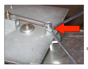
REMOVE PLUNGER SPRING AND PLUNGER BOLT AT END OF FEEDER TRAY. INSERT SCREW THROUGH HOLE AT END OF SAFETY RING HOLDING RODS BETWEEN THE TWO NUTS ON BOLT, SECURE AND ADJUST RODS.
