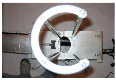
Safety Ring Guard shows the projection of the throwing arm when in use to ensure safety.
