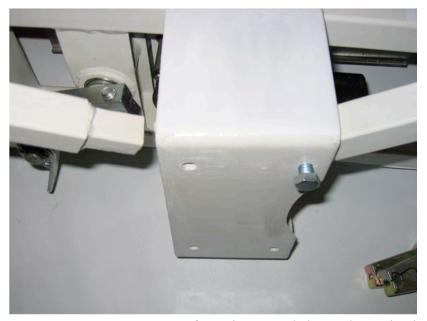
Attach each short pole ensuring that the smaller poles are in the front of the trap and larger poles are in the rear. Line up horseshoe with top of the poles screw in long poles through horseshoe into short poles. Now attach horseshoe to top of poles and tighten hex screws.
