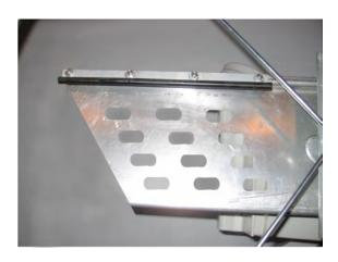
Because the clay lands directly onto the throwing arm, the Aerial Assault needs little adjustment. Loosen the two bolts on either side of the trap to adjust your throwing angle. Once desired angle is reached, tighten bolts back.
