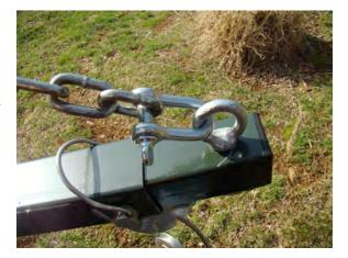
**5.** Attach remaining clamp to o-ring at end of hoist arm and use it to attach other end of shorter chain to hoist at desired length and angle.
