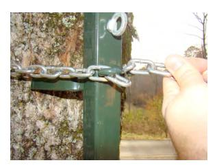
3. Attach one end of the longer chain to hook at the top of hoist. Wrap chain around the tree and secure link of chain to the other hook at top of hoist to hold hoist firmly to tree.
