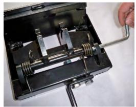
3. Resting spring arms on top of the back bar on base, align support brace barrel with holes on base and insert the L-shape pin.
