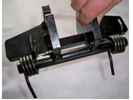
2. Insert two springs onto the ends of barrel on support brace, paying attention to the angle and position of the springs. Spring arms should rest on top of support brace "wings".
