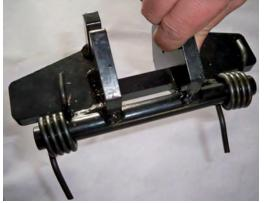
2. Insert two springs onto the ends of barrel on support brace, paying attention to the angle and position of the springs. Spring arms should rest on top of support brace "wings".
