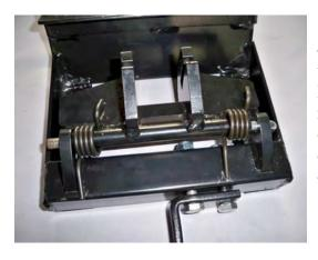
4. Make sure the handle of L-shaped pin is pointing down so it can only be pulled out by hand.
