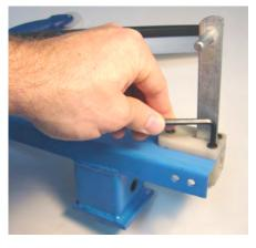
Attach Trigger by separating the 2 parts of the trigger block. Slide trigger facing up into slot in the back of the trap head with the small part of the block on top of the trap head and the large piece below. Tighten the bolts securely through the block using the nuts underneath.
