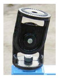
Attach pivot mount to unit frame – Attachment will be the same regardless of type (ie: Post Mount, Clayhawk, Single or Double.
