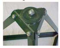
Take the 1 3/4" hex bolt and push up through the center hole of the Triangular/Top Pivot casting securing with the 1/2" hex nut. This is where you will attach the 3 Pivot Mount and your Trap Head.
