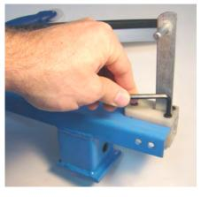
Attach Trigger by separating the 2 parts of the trigger block. Slide trigger facing up into slot in the back of the trap head with the small part of the block on top of the trap head and the large piece below. Tighten the bolts securely through the block using the nuts underneath.
