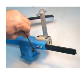
Attach handle to inside of trap head by screwing allen bolts through trap head into handle. Tighten securely.
