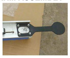
Place the paddle-shaped counter balance on the arm, aligning all pre-drilled holes. By using the allen screws, attach the throwing arm and counter balance to steel mounting plate and secure tightly with provided allen wrench.
