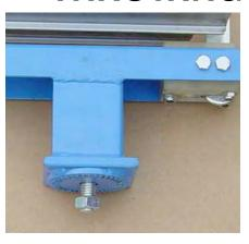
Insert 1 3/4" bolt into hexagon shaped opening, in the trap head carriage through the top of the pivot mount assembly; interlocking the gear mesh teeth. Secure with 1/2" nut using wrench.
