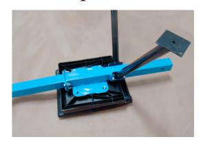
Take plastic seat and position onto the seat plate/seat assembly making sure the seat back folds toward the flat mounting plate for the tail beam assembly. Secure the seat to the seat plate by using the 4 self tapping screws.
