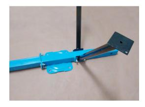
Take the four support legs and slot them into the four leg brackets as per pictures. \*\*\*\*\*\*Note that the predrilled holes at the end of each leg are the feet not the mounting brackets. These holes are provided if you want to mount your trap frame to a solid surface or platform.
