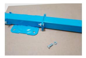
Take the tail beam and assemble securely to the flat mounting plate on the back of the seat assembly using four 3/8" nuts and 3/8" bolts.
