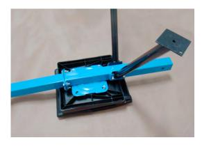
Take plastic seat and position onto the seat plate/seat assembly making sure the seat back folds toward the flat mounting plate for the tail beam assembly. Secure the seat to the seat plate by using the 4 self tapping screws.
