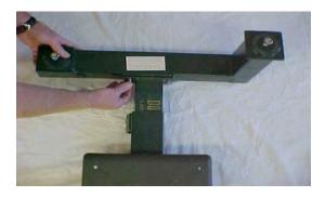
Take the tail beam and assemble securely to the flat mounting plate on the back of the seat assembly using four 8M nuts and 8M bolts.
