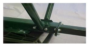
Take the two long/rear support legs and slot them into the two rear leg brackets. Note that the predrilled holes at the end of each leg are the feet not the mounting brackets. Therefore they should be the end that will be sitting on the ground. These holes are provided if you want to mount your trap frame to a solid surface or platform.
