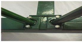
Take the two short/front support legs and slot them into the two front leg brackets under the Front T Tube. Note that the predrilled holes at the end of each leg are the feet not the mounting brackets. Therefore they should be the end that will be sitting on the ground. These holes are provided if you want to mount your trap frame to a solid surface or platform.
