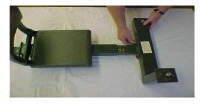
Place the seat assembly/sliding beam assembly upright (with plastic seat on top). Take the Front T Tube and place it against the mounting plate at the front of the sliding beam assembly. With the four holes alligned, screw in the four 3/8" Bolts into the the threaded holes on the Front T Tube.
