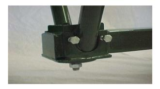
Take the four support legs and slot them into the four leg brackets as per pictures. Note that the predrilled holes at the end of each leg are the feet not the mounting brackets. Therefore the square plates with holes should be the end that will be sitting on the ground. These holes are provided if you want to mount your trap frame to a solid surface or platform.
