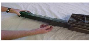
Place the seat assembly upright (plastic seat on top) and slide the Sliding Beam Assembly into the seat assembly to desired length and then lock into position with two 3/8" bolts.
