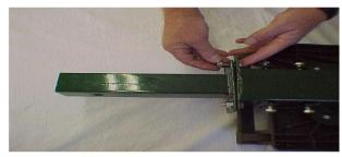
Take the tail beam and assemble securely to the flat mounting plate on the back of the seat assembly using four 3/8" nuts and 3/8" bolts.
