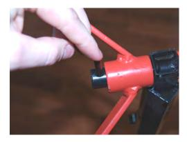
4. The Left and Right Target can go on either side, so there is no designated left and right target, either will work. Take one of the targets and slip it on the Top Target Axle. You will notice a hole in each one of the Axles. This is where you will hammer in the 2 Roll Pins that are provided. The 2 Roll Pins don't have to go all the way down, just hammer so they are equally through on the top and bottom of the Axle.
