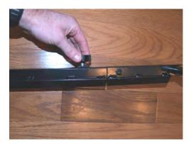
**2.** Use the provided Thumb Screw and tighten the Base Extension and the Top Target Axle together.
