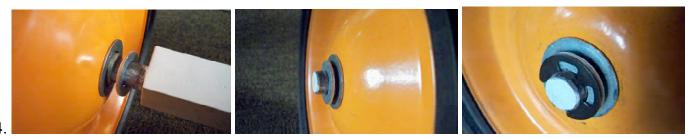
Assemble two wheels. Slide spacer over axle then attach the wheel onto axle, then insert another spacer on outside of wheel. Finally attach locking washers to outside of the wheels.
