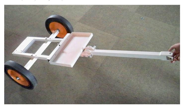
Remove bolt from tabs at base of pulling arm. Pull out back long bolt from posts to allow the arm to swing down into straightened position. Replace long bolt though the posts and arm to lock the arm straight. Remove handle from end of arm and secure it to post in front of battery tray with spare nut. Use bolt and nut from handle to secure arm to back of ATV.
