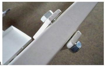
Insert handle between prongs at end of pulling arm, attach with M10X60 bolt and nut. (When pulling with ATV, you will remove this handle.)
