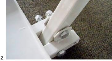
To attach pulling arm: Insert end of arm between posts behind battery tray. Insert M10X50 bolt to attach arm between tabs locking with nut on other side. Insert M10X95 (long) bolts into posts, locking on the other side with nuts. Bolt closest to battery tray should go through the arm. Back bolt will be used to lock arm in straight position if limo is going to be pulled by an ATV.
