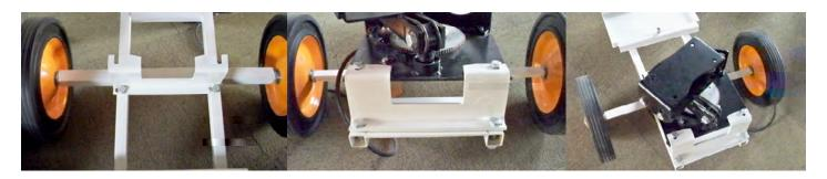
Using M10X45 bolts attach first bracket to front of trap platform then place the base of the AWK45 under the curved edge of the bracket and tighten the two bolts on the AWK45. then attach second bracket to the holes behind the axle and tighten the two bolts on the back of the AWK45 wobbler kit tightening them to the back bracket. Follow Wobbler Kit instructions to attach trap.
