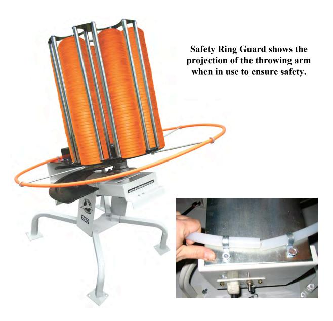
TO ASSEMBLE: ATTACH 3 HOLDING ARMS UNDERNEATH DECK OF THE TRAP USING THE 3 SCREWS ATTACHED TO THE DECK. LOOSEN CLAMP BOLTS ON REAR OF TRAP AND SLIDE EACH END OF THE PLASTIC GUARD AS SHOWN ABOVE. REMOVE ONE OF THESE BOLTS TO INSERT THE END OF SAFETY PIN CHAIN UNDER BOLT TO SECURE YOUR SAFETY PIN TO THE TRAP.
