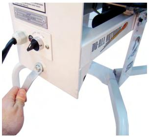
Loosen the bolts on either side of the trap to adjust the throwing angle. Once desired angle is reached, tighten the bolts.
