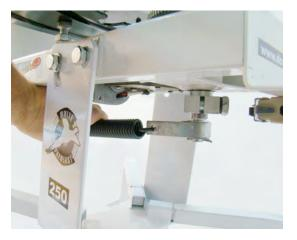
Rotate arm counter clockwise to 12:00. Insert Black Main Spring into silver swiveling spring hook. Attach Spade Bolt to spring & feed thru opening at back of trap. Tighten to show 1 or 2 threads on the back side of the lock nut. Now tighten the inner lock nut closer to the frame.
