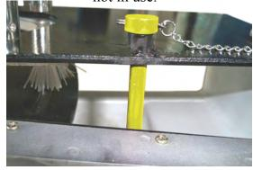
This pin is designed to catch the arm, the trap should be disarmed and the spring disconnected if transporting, working on, adjusting or storing.
