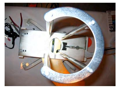
Safety Ring Guard shows the projection of the throwing arm when in use to ensure safety. TO ASSEMBLE:
