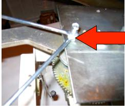
REMOVE PLUNGER SPRING AND PLUNGER BOLT AT END OF FEEDER TRAY. INSERT SCREW THROUGH HOLE AT END OF SAFETY RING HOLDING RODS BETWEEN THE TWO NUTS ON BOLT, SECURE AND ADJUST RODS.
