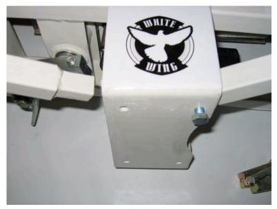
Attach each pole ensuring that the smaller poles are in the front of the trap and larger poles are in the rear. Now attach horseshoe to top of poles and tighten hex screws.
