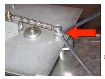
REMOVE PLUNGER SPRING AND PLUNGER BOLT AT END OF FEEDER TRAY. INSERT SCREW THROUGH HOLE AT END OF SAFETY RING HOLDING RODS BETWEEN THE TWO NUTS ON BOLT, SECURE AND ADJUST RODS.
