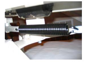
Rotate arm counter clockwise to 12:00. Insert Black Main Spring into silver swiveling spring hook. Attach Spade Bolt to spring & feed thru opening at back of trap. Tighten to show 1 or 2 threads on the back side of the lock nut. Now tighten the inner lock nut closer to the frame.
